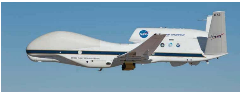
1. The Global Hawk is a high-altitude UAV that has shown the endurance to remain in flight for 30 hours continuously. (Courtesy of Northrop Grumman)
