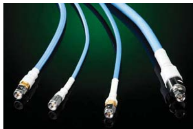
4. Standard PhaseTrack cables and cable assemblies incorporate a proprietary dielectric for high phase stability over temperature. A cable with a 0.108-in. diameter has a cutoff frequency of 80 GHz. (Courtesy of Times Microwave Systems)
