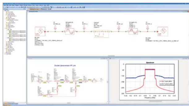
1. Rohde & Schwarz and Cadence cooked up a signal creation and analysis tool that hastens the development process for RF components.
