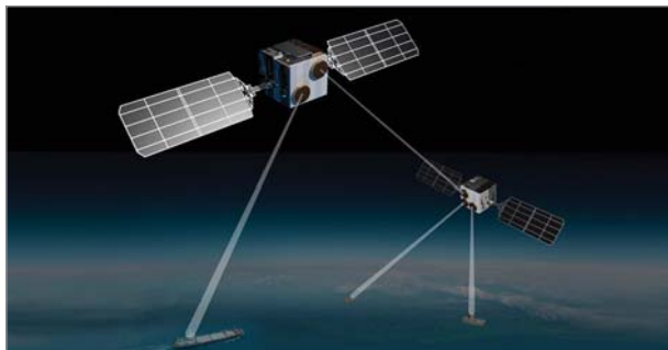
3. ThinKom Solutions' compact, lightweight antennas serve inter-satellite, Earth-to-space, and space-to-Earth links while supporting nesting and beamforming.
