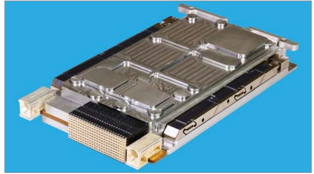
10. Mercury Systems' RH3480 SSDR is SWaP-optimized to provide 480 GB of industrial-grade memory in a 3U VPX-compatible enclosure weighing only 750 g.
